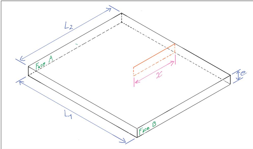
The figure shows a rectangular part (representing the Aluminium coating). The electrical resistance is measured between Face A and Face B. The crack (shown in orange) has a length of  $x$ , while the coating has dimensions of  $L_1$ ,  $L_2$  and  $e$  (thickness). We will assume that the speed of electrical signal (speed of light order) is way faster than the speed of propagation of the crack (a few km/s). We hence can say that only  $x$  impacts the resistance, and not  $dx/dt$ .
